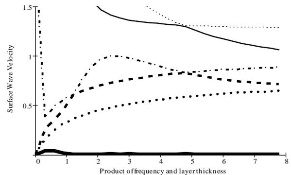
**Figure 3.** Dispersion curves for the first six modes of thermoelastic waves propagating modes in layered structure consisting of the upper layer from material I and the substrate material II with thermal relaxation time  $\tau_0 = 4.0 \times 10^{-6}$
