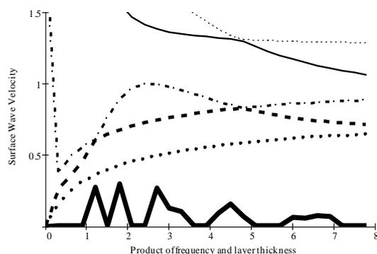
**Figure 1.** Dispersion curves for the first six modes of thermoelastic waves propagating modes in layered structure consisting of the upper layer from material I and the substrate material II with thermal relaxation time  $\tau_0 = 4.0 \times 10^{-8}$
