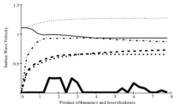
**Figure 4.** Propagating modes in layered structure consisting of the upper layer from material I and the substrate material II when thermal coupling constant equal to zero
