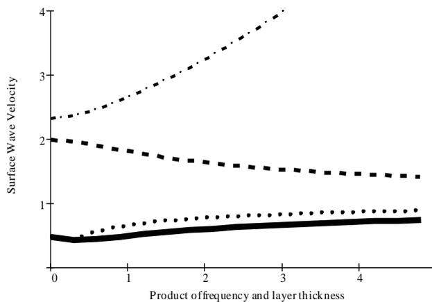
**Figure 5.** Dispersion curves for the first six modes of thermoelastic waves propagating modes in layered structure consisting of the upper layer from material I and the substrate material II when thermal relaxation time is zero
