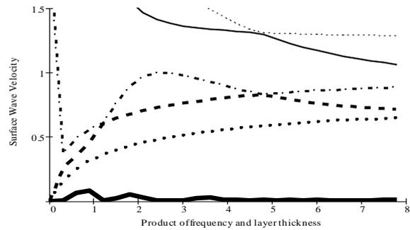
**Figure 2.** Dispersion curves for the first six modes of thermoelastic waves propagating modes in layered structure consisting of the upper layer from material I and the substrate material II with thermal relaxation time  $\tau_0 = 4.0 \times 10^{-7}$
