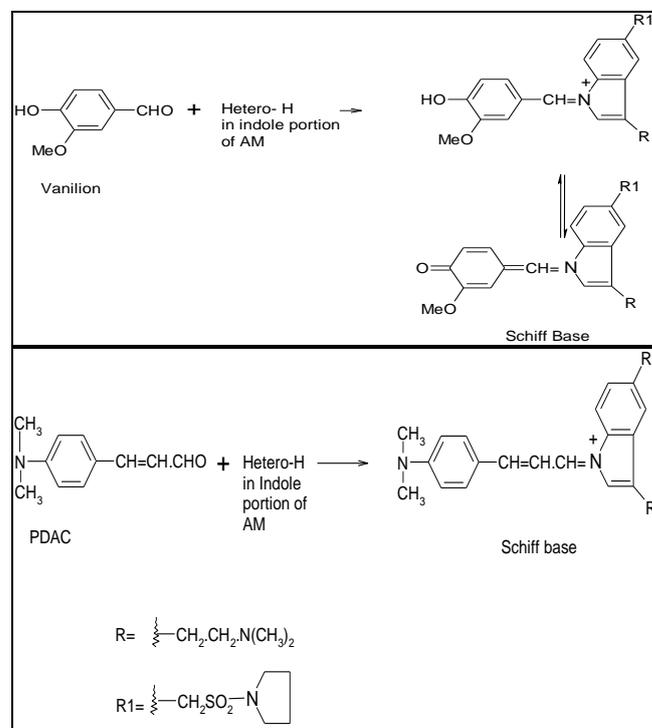
**Figure 6.** Scheme of reactions
