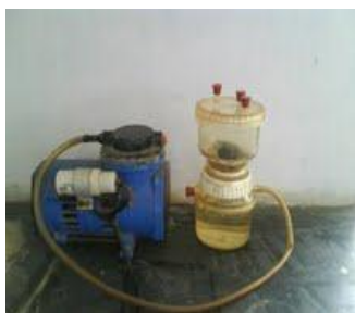
Figure 4. Filtration of the Enzyme (Lipase) Using Millipore Filter
